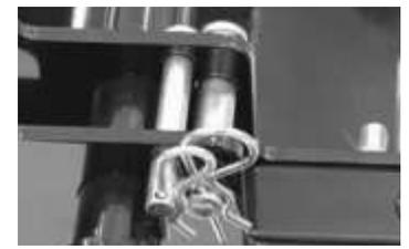
Extra Pin Storage at each end of machine by axle.
