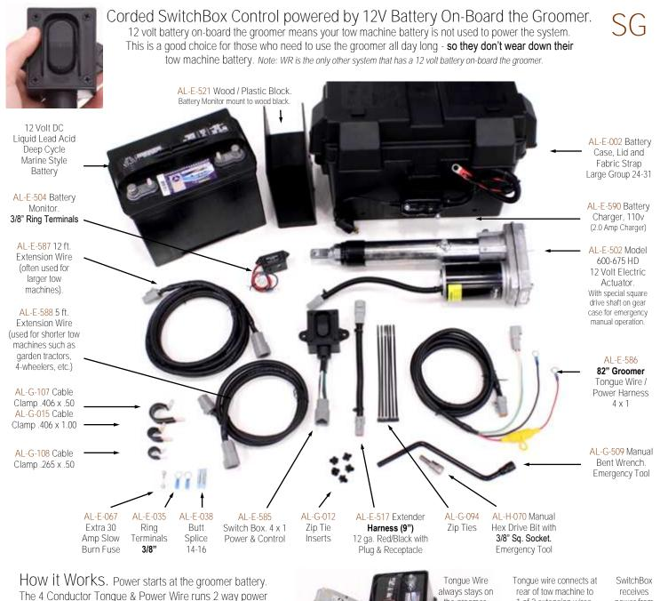
HOW IL WOLKS. Power starts at the groomer battery. The 4 Conductor Tongue & Power Wire runs 2 way power towards the operator (through whichever extension wire is used) and onto the SwitchBox. From switch 2 way control is returned to the actuator on groomer.
