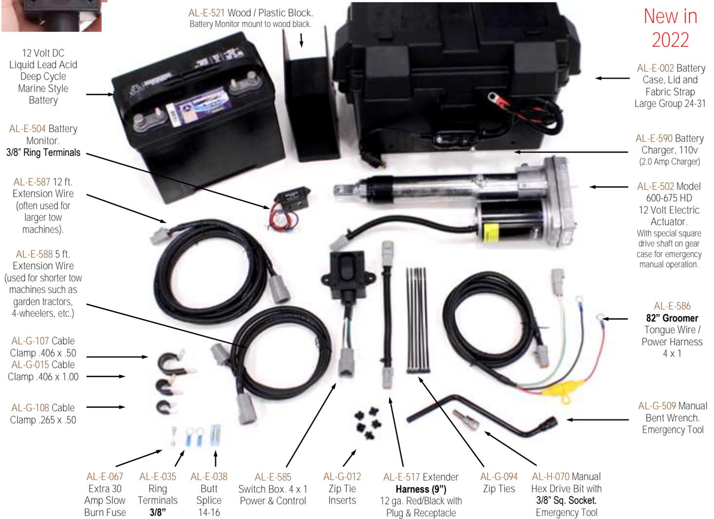
**How it Works.** Power starts at the groomer battery. The 4 Conductor Tongue & Power Wire runs 2 way power towards the operator (through whichever extension wire is used) and onto the SwitchBox. From switch 2 way control is returned to the actuator on groomer.
